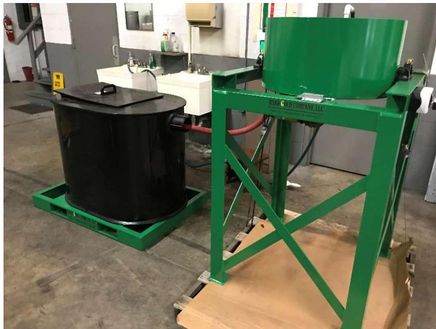
Prototype FOWA showing Green Reaction vessel connected to an Oil Water Separator (Black) through bottom drain
